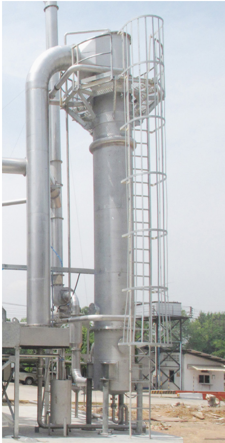
Shell & tube condenser at ASTW fish meal plant in Thailand
